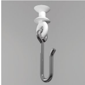
SLIDE CARRIER CE7019 Available in packs of 10 only. Peak load: 51.7 lb(f) (23kg(f)) Carrier Height: 2" (51mm) Wheel Height: 5/16" (7.9mm)
