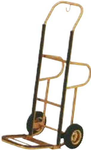
Model# Finish HT-1B Brass Size: 15" L x 15" W x 48" H Constructed with 1" Tube 8" Pneumatic Wheels
