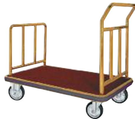
Model# Finish FB-1B Brass FB-1C Chrome Size: 42" L x 24" W x 36" H Constructed with 1 1/2" Tube, 6" Solid Wheels Red Carpet Bed & Bumper Guards
